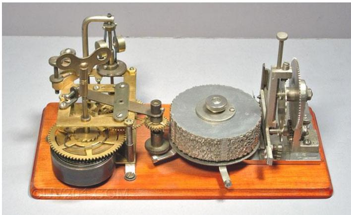
*The basic Omnigraph model used only a single code disk. This severely limited the length of the recorded code pattern, and students could cheat once they memorized what was on the disk.*
